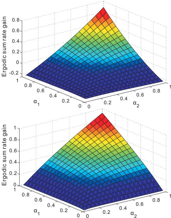
Figure 3. Ergodic sum rate gain  $((R_{Co} - R_{Non-Co})/R_{Non-Co})$  vs. RNs' activation probability  $(\alpha_1, \alpha_2)$  for: scenario a),  $H_a$  (upper plot) and scenario c),  $H_c$  (lower plot).
