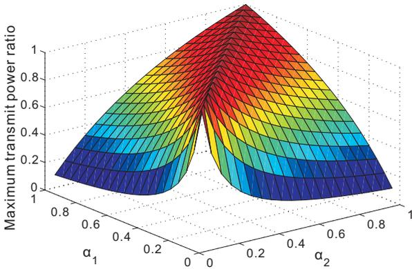
Figure 4. Maximum instantaneous transmit power ratio  $(P_{Co}^{\max}/P_{Non-Co}^{\max})$  vs. RNs' activation probability  $(\alpha_1, \alpha_2)$  for scenario a),  $H_a$ .
