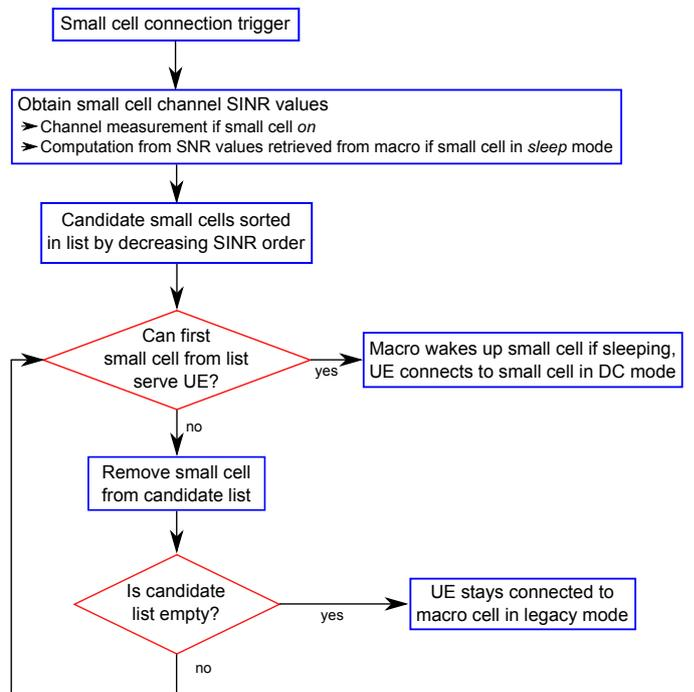
Figure 3. Flow chart representing the *maximum SINR* connection principle
