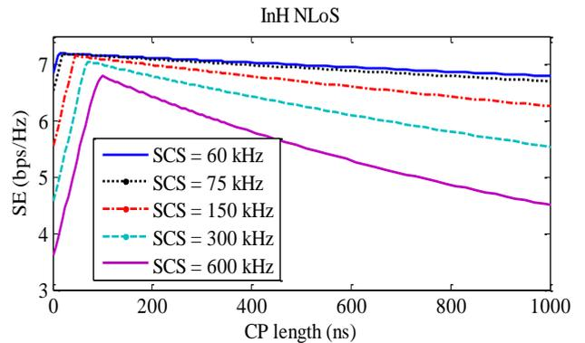
Fig. 2. Spectral efficiency as a function of CP length for InH.
