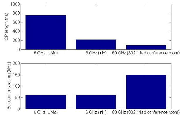
Fig. 5. Optimal CP length and subcarrier spacing.
