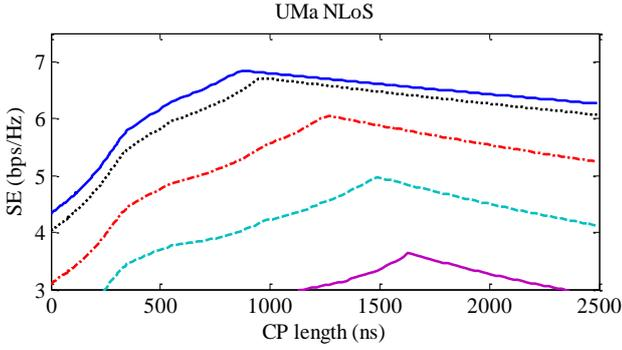
Fig. 3. Spectral efficiency as a function of CP length for UMa.
