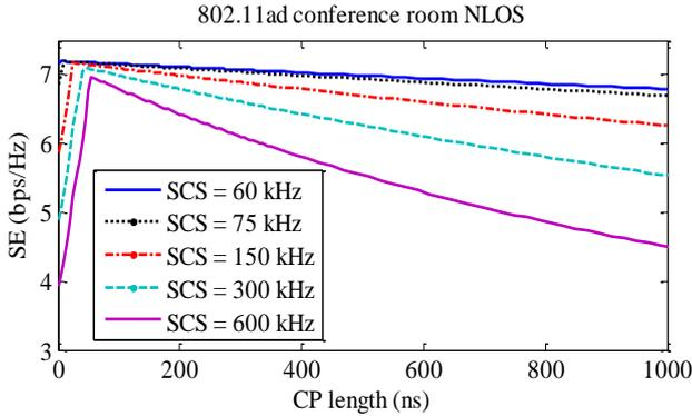
Fig. 4. Spectral efficiency as a function of CP length for 802.11ad conference room.
