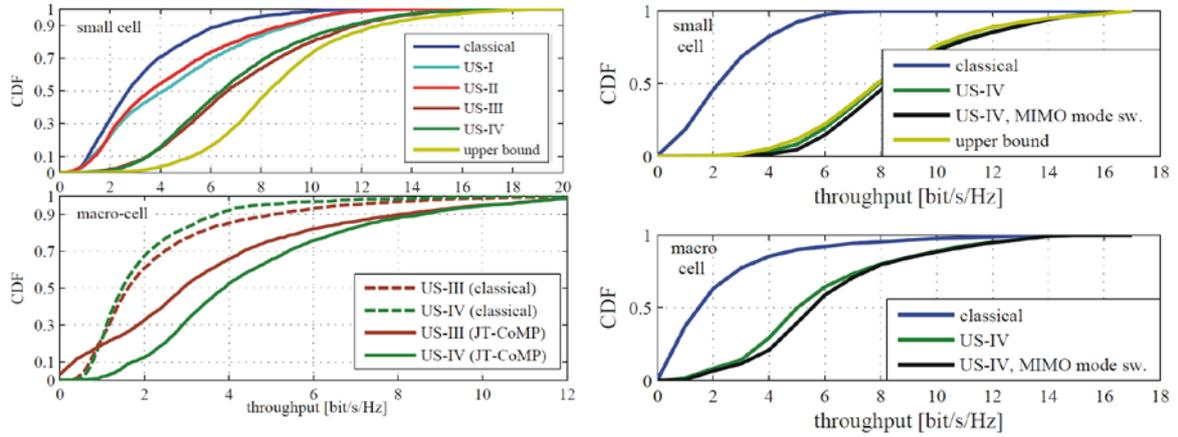
Fig. 1 Left: User throughput in a small cell and in surrounding macro-cells. Right: Optimized performance after rank adaptation and frequency-selective scheduling.
