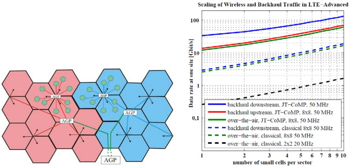
Fig. 4 Left: Model of a heterogeneous mobile network including triple-sectored macro-cells and embedded small cells. Backhaul is organized as a tree using a switch at each aggregation point (AGP). Right: Scaling of mobile data and the corresponding backhaul traffic versus the number of small cells.
