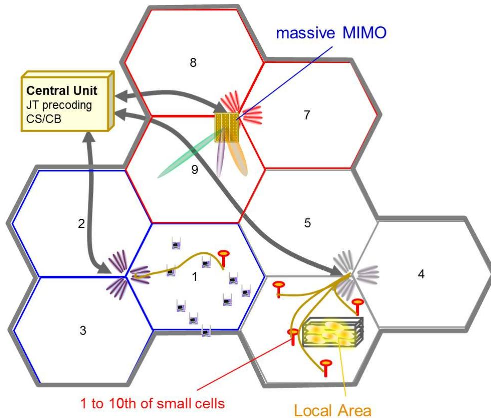
Figure 3: 5G system concept enhancing 4G systems by adding small cells, massive MIMO and JT CoMP for interference mitigation. Interference floor shaping is assumed to overcome inter-CA interference.
