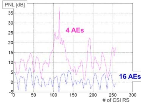
Figure 3: Power normalization loss of ZF precoder serving 3 UEs with 4 and 16 columns of antennas. Each antenna has eight vertical antenna elements, i.e. overall there are  $8 \times 16 = 128$  elements.
