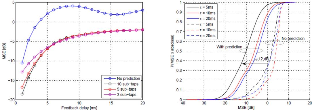
Fig. 2 Left: Average precision of the CSI versus the feedback delay with and without prediction, assuming perfect CSI at the terminal at 30 km/h. The oscillation with no prediction is due to the temporal correlation in the SCME channel. Right: For typical values of the delay, CSI precision can be increased.
