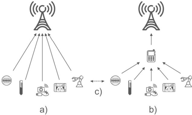
Fig. 2. HT MMC illustrated in the case of a) direct access, b) accumulation point access, and c) M2M access.
