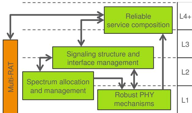
Fig. 5. Toolbox of generic mechanisms for URC and their interactions.
