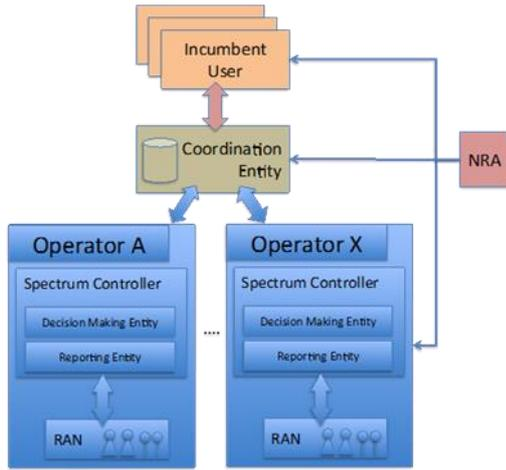
Fig. 1. Spectrum Sharing Functional Architecture
