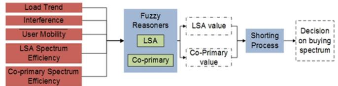
Fig. 2. Fuzzy Logic based Spectrum Controller
