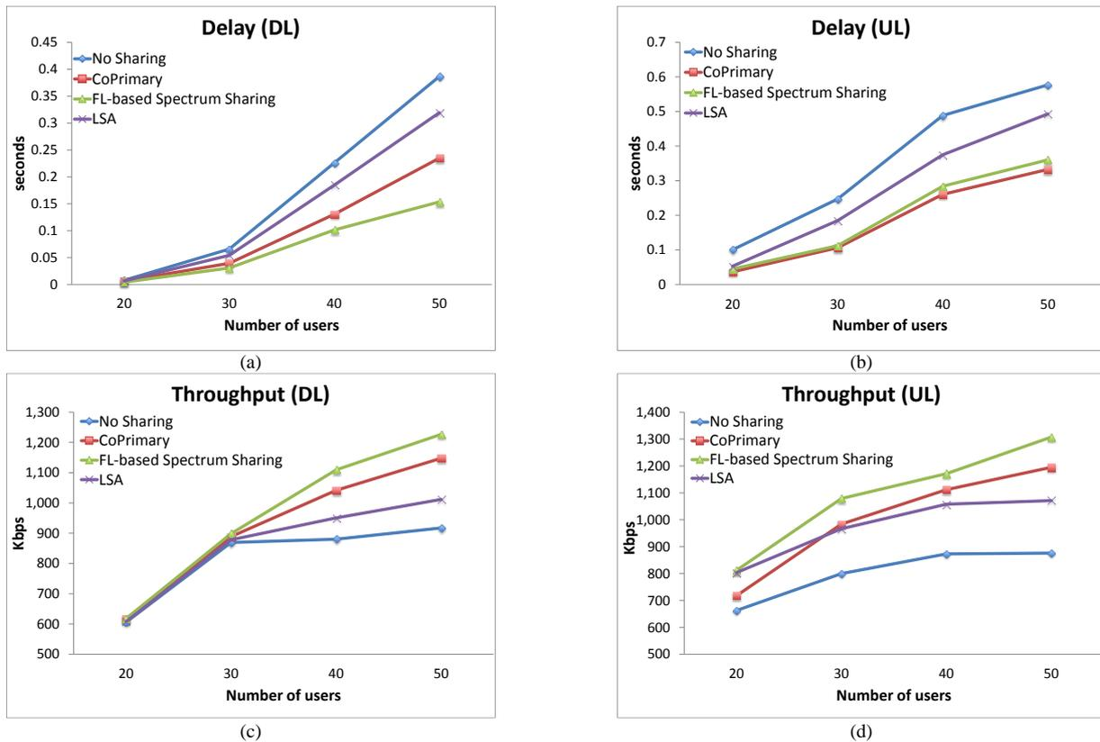
Fig. 3. Simulation results for 20, 30, 40 and 50 users. (a) Downlink Delay, (b) Uplink Delay, (c) DL Throughput, (d) UL Throughput
